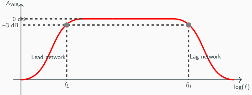
Figure 5: A typical Gain versus Frequency or Bode gain plot
